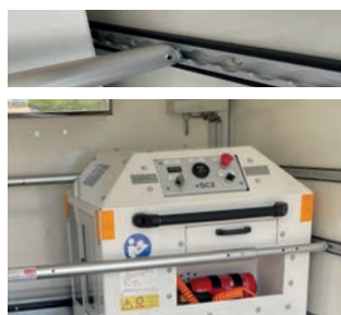
Image: Trailer with fixing system, socket strip and LED light rail
